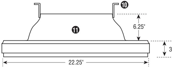
**CURB MOUNTED FLASHING**
